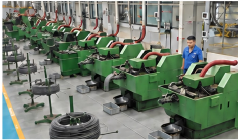
FASTENER PRODUCTION / COLD HEADING & THREAD ROLLING
